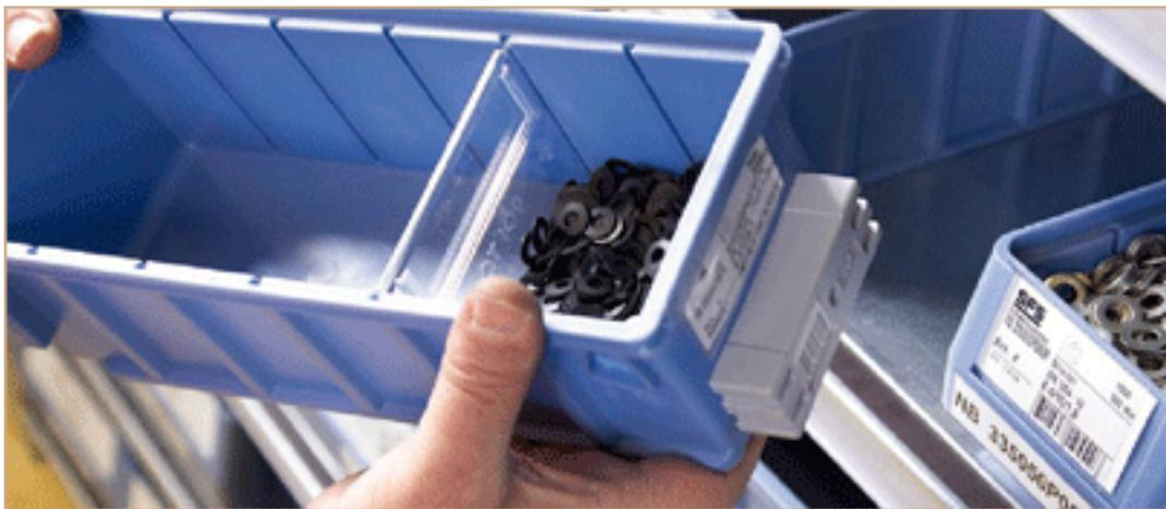
*Each parts container is fitted with an active RFID tag.*
